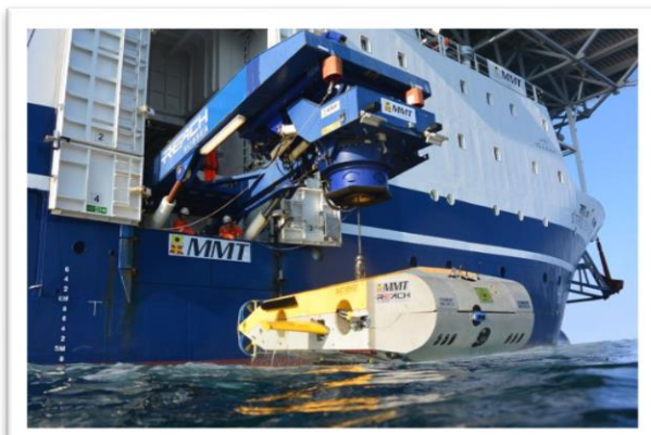
The Remotely Operated Vehicle (ROV) Surveyor Interceptor. It flies at 4-6 knots, 3-4 times as fast as conventional ROVs. It carries multibeam and sidescan sonar, sub-bottom profiler, HD cameras, powerful lights and a laser scanner. It was Black Sea MAP’s principal survey tool in 2016 and operated at depths down to 1800m (over a mile down). Photo credit: MMT
