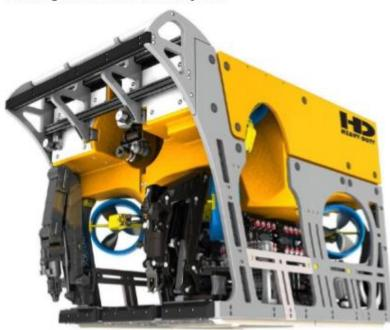
Havila Subsea are equipped with 2 x Schilling Robotic HD WROV systems. The HD™ WROV is a 150hp, compact remotely operated vehicle that is designed for accommodating the specific needs of the IMR and drill support markets. The HD™ system is optimized for installation onboard drilling rigs and ROV support vessels, where available deck space is limited.
